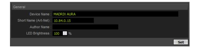
**Device** Allows you to change the main label of the device by entering a name. The default setting is **Name** MADRIX AURA.
