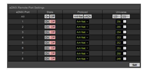
**eDMX Port** 8 individual ports, i.e. universes, are available for remote control over Art-Net or Streaming ACN.
